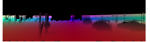
(b) Projected and up-sampled LiDAR points into the camera frame
