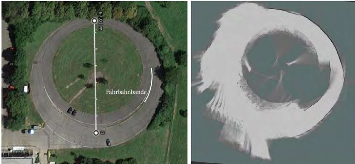
Fig. 3. Exemplary occupancy grid map of the Offenburg test track, based on LiDAR, inertial and odometry sensors.
