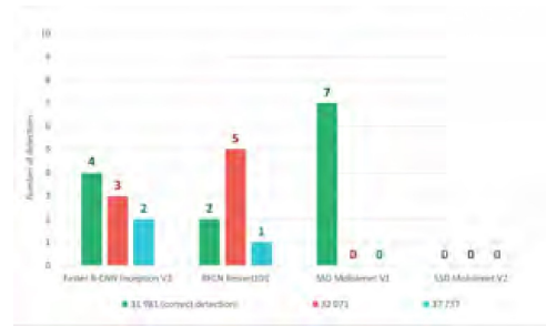
Fig. 6. Overview of the behaviour of different neural networks when detecting parts with strong similarity using the example of detections in images of part 31 981.
