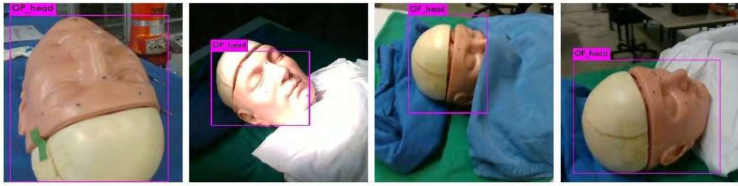
Fig. 8. Coarse determination of the patient's head on the OR table with YOLO v3.
