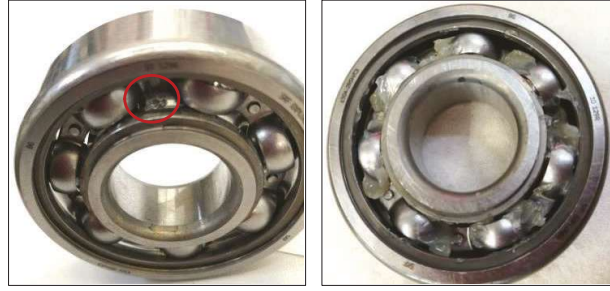
Fig. 2. Example of engraved spall in the inner-ring (left) and example of reduced amount of lubrication for measurement (right)
